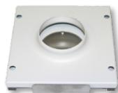
5. Verify the intake and exhaust vents are closed. Both vents **must be closed** for an accurate calibration.
