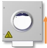
**3.** Secure the reference temperature device sensor probe at the center of the middle shelf, with the probe head 2 inches above the shelf surface.
