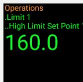
Use the **Set the High Temperature Limit** procedure on page 29 to set the Limit heating cutoff to at least 10°C above the highest intended temperature of your application.
